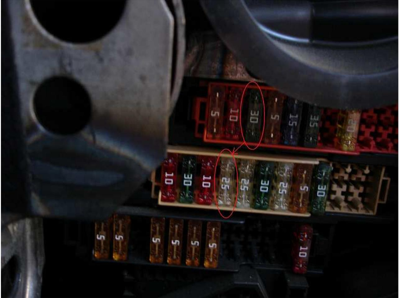
If you are still not able to get communication with the ECU it is possible to make short of the external fusebox (it is found under the front cover, where the engine is). You have to short the first 5A fuse with the +12V connection as shown on the picture. Please pay attention that you have to use a bigger cable because if you use a small cable it can heat up.
